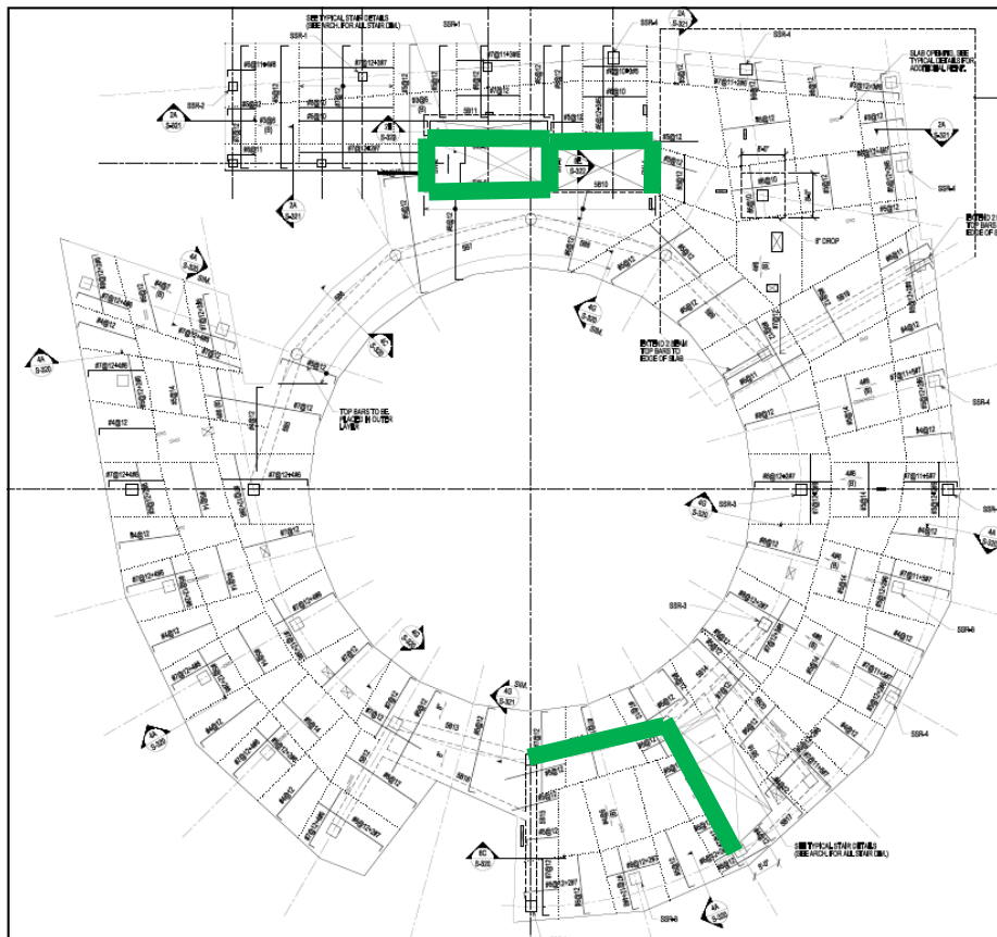
Figure 3: Shear wall locations. Courtesy of RTKL.
